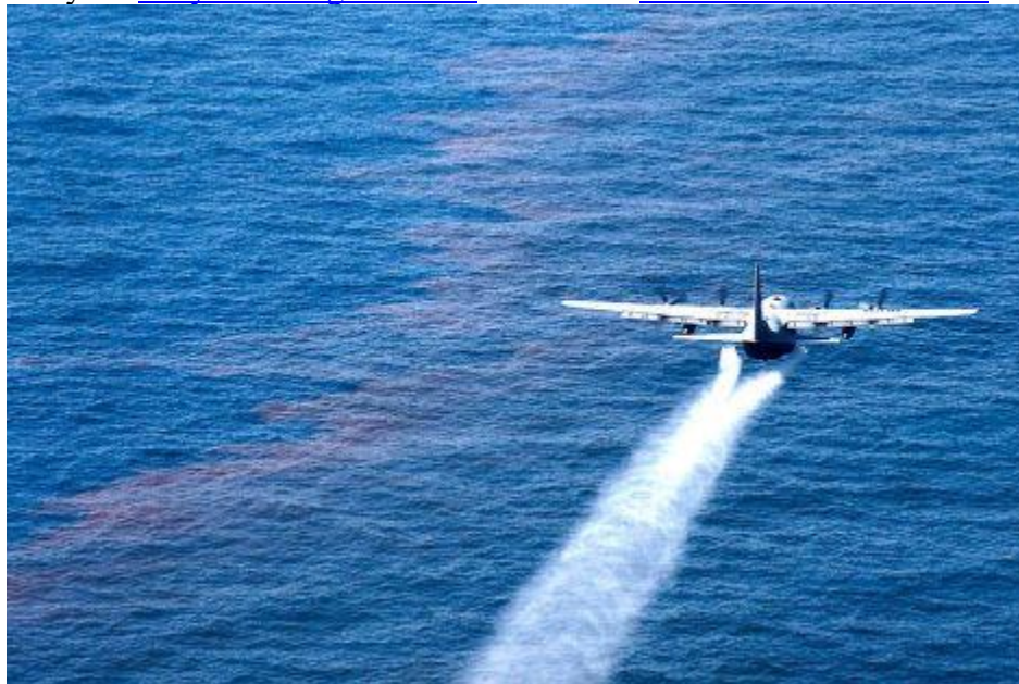
U.S. Air Force A C-130 Hercules sprays Corexit onto the Gulf of Mexico.
